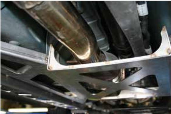
The center section should be installed as high as possible to maximize ground clearance, but low enough to clear the exhaust pieces. Remember that your exhaust parts are on rubber hangers and they will move around! Once you've determined the correct height, tighten up all the bolts. You can raise a sagging exhaust system by installing new hangers or using a hose clamp around the existing hangers to tighten them up.
