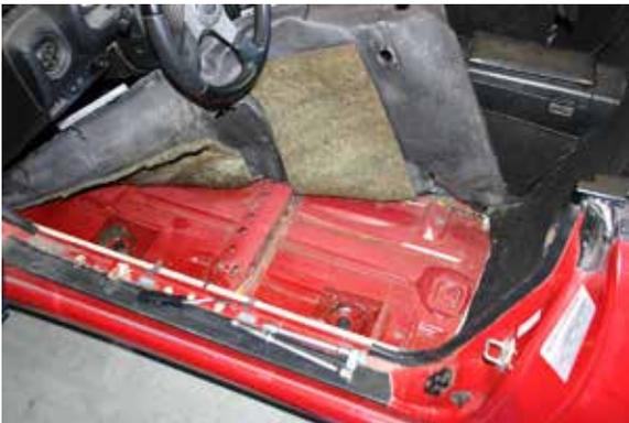
This installation can be done fairly easily, although it will take a bit of time. Tools required will be a drill with a 5/16" bit, a screwdriver, and sockets / wrenches. We recommend you wear gloves when handling these pieces as they have sharp edges.
