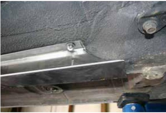
1/2" or so too far rearward, the rearmost bolt hole will go into the bulkhead! Do the same steps to square both rails up equally before drilling any holes in the floor pan. It is very important to get both sides square so that if you're adding the Butterfly section (available as a package or separately) it will bolt directly up.
