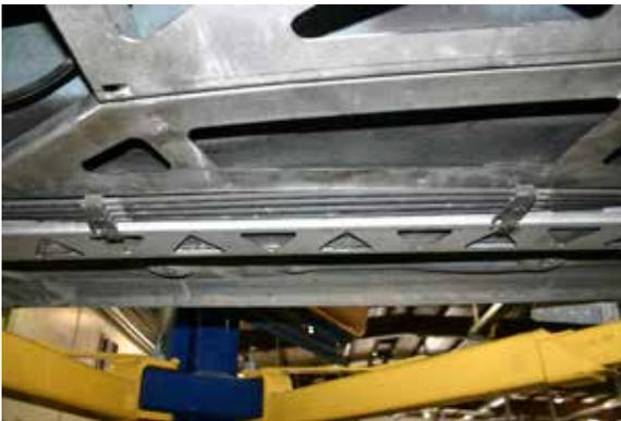
The brackets for the fuel lines need to be bent for re-installation (when the job is complete) as shown in the photos. Slip the brackets over the studs in the right hand frame rail and tighten down the supplied nuts (not shown in the pictures). The fore and aft floating brackets can be attached per the photos below as a buffer between the rail and the fuel lines.
