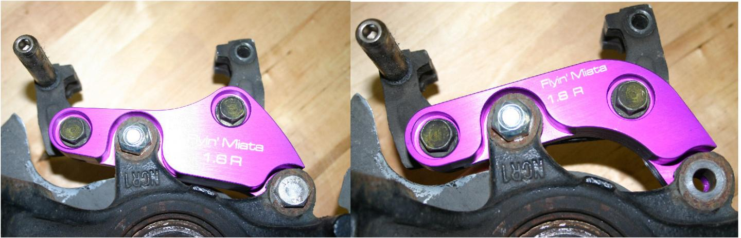
9. Slide the stock bracket over the rotor and bolt it onto the upright. Use the stock hardware here. Tighten both of these to 36 ft-lbs, using Loctite.
