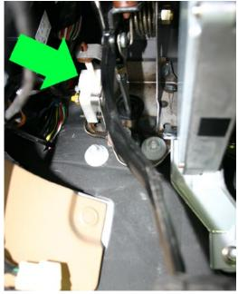
Installation of the clutch switch override should only take a few moments, but it is awkward. No tools are required. Keep in mind that once the override is installed, your Miata will start even if it is in gear. Always make sure the car is in neutral before trying to start the car.
