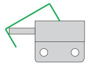
The override clip will slip over this switch, sitting on top. It's shown in green in the diagrams. Hook one end of the clip over the plunger on the switch as shown, and hold it in place with your thumb.
