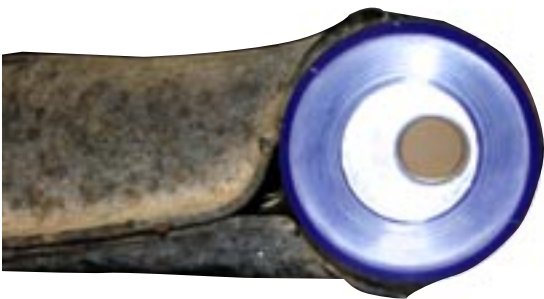
Bushing set for more negative camber
