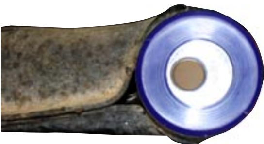
Bushing set for more positive camber
