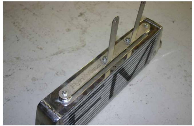
Note the position of the Flyin' Miata engraved in the lateral bar. In this case, the painted FM on the intercooler will be facing forward. Use the two M8 x  $1.25 \times 16$  mm (36-10420) bolts to attach the assembly to the top of the intercooler. The outlets are at the bottom. The intercooler is symmetrical so it can be installed to make the painted FM visible through the grille (as shown) or facing the radiator.
