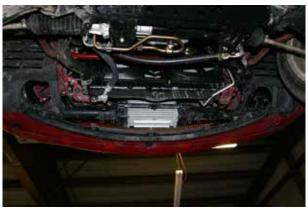
Installation of the new intercooler is relatively straightforward. The stock steel intercooler pipes will have to be cut in order to accomodate the larger piece, however. Tools required are a 8, 10 and 14mm wrenches, a Philips screwdriver, big pliers and some way to cut the pipes.
