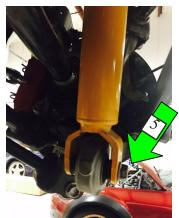
Access the rear upper shock mounts by removing the felt trunk liner. There are several plastic clips holding the liner in place. Remove them by first pulling up the center section to release the clip. Then gently remove them by pulling on the outer section. Again, remove the two large nuts holding the mount in place, **NOT** the center nut.
