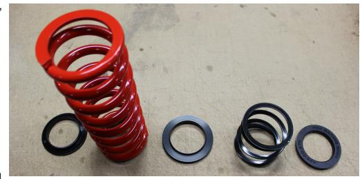
on shaft), spacers (see information next page), large washer (concave face points up towards bushing, same as the gold one at the top), stepped bushing (shoulder points up towards shock mount), shock mount, stepped bushing (shoulder points down towards shock mount), large washer (concave face points down towards
