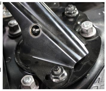
hole where the grease is on the brace. Bigger is typically better here, in case the hole isn't centered. Repeat for the other side. The adjustment knob can manipulated from the backside, by rolling your finger over it.
