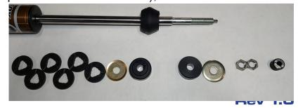
Torque the first nut to 10 lb-ft, then tighten the second nut against the first nut while holding the first nut stationary. Be sure the set screw on the adjuster is lined up with the flat on the shaft, then tighten the set screw in the adjuster.
