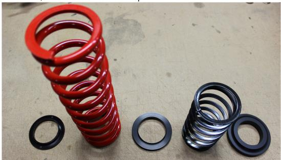
• The shock mount assembly is the same as well. Again, from left to right: bump stop (shown on shaft), spacers, large washer (concave face points up towards bushing), stepped bushing (shoulder points up towards shock mounts), stock shock mount
