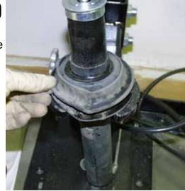
orientation and not "quite right" in the other orientation. If you have the rubber bushing at the base of the factory shock, install it on the new shocks as shown. If you don't, don't worry about it - it's not a critical piece.
