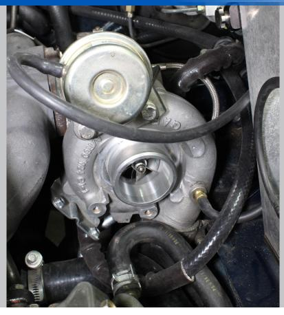
This kit is intended to work with our FM coolant reroute kit, allowing you to reroute the turbo water so that the engine as a whole runs cooler. It's a simple install, but be sure to route the lines carefully. If you have any questions or suggestions for improvements, please don't hesitate to get in touch with us.
