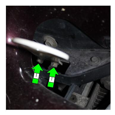
2. The rear hook (29-99001) installs in the same manner, replacing the right rear tie down point (it won't work on the left side). The rear hook isn't indestructible, but it's stronger than the front hook. The rear hook only works for 1990-1997 cars.
