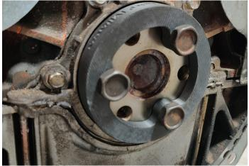
what the tool is for), just push it up until it contacts the seal retainer. Slip the tool over the end of the shaft, and use the original bolts (that hold the flywheel on) to press the tool (and hence the seal) into place.
