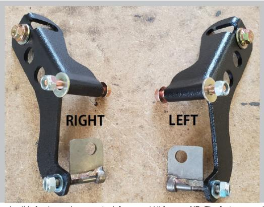
Thanks for purchasing this front sway bar mount reinforcement kit for your ND. The factory sway bar brackets on the ND are inherently weak. These brackets strengthen the subframe to prevent fatigue and failure. These brackets are especially important on cars with sticky tires and aftermarket sway bars. If you have any questions during installation or suggestions for improvement to the product or the instructions - please don't hesitate to call or email.
